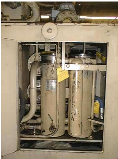
Short housings showing flat housing cap mod, and a 20" filter housing.
